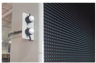
Figure 1. Media Resources standard - dual ambient brightness measuring photocells for hardware redundancy
