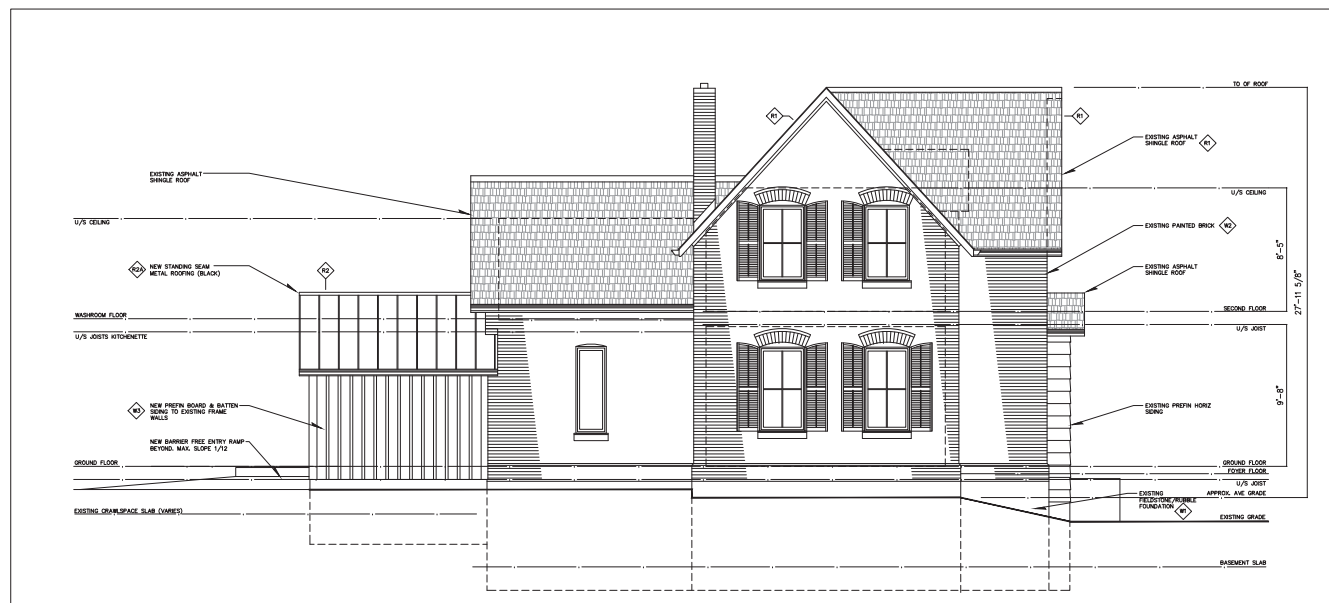
2 A3.2 NORTH ELEVATION - EXISTING TO REMAIN - NEW B&B SIDING TO EAST END 1/4" = 1'-0"
