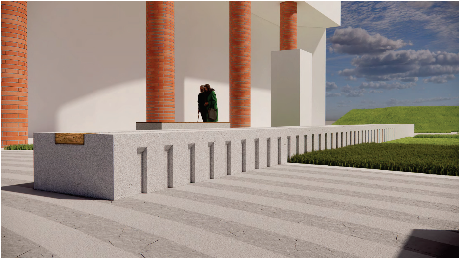
Image of "Sky Ribbon" Plinth depicting simple formwork impression that fades as it grows further from the Gathering Place. Note: Vegetation removed to show relationship to adjacent spaces.
