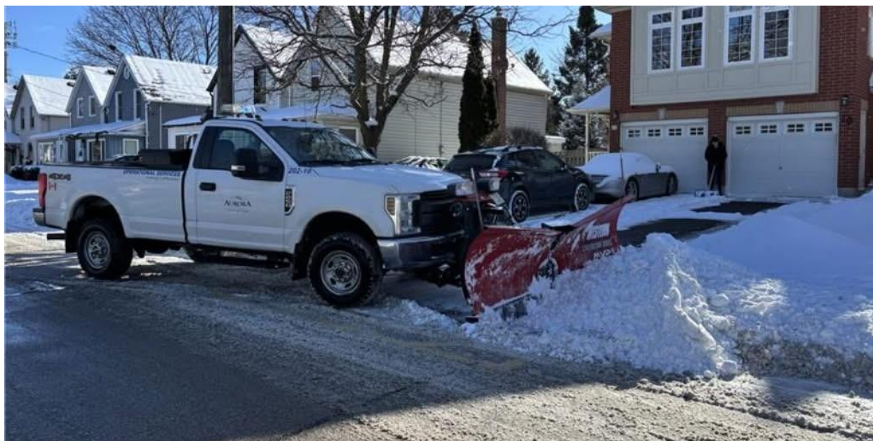
Figure 2: Shared driveway windrow removal reverse truck.
