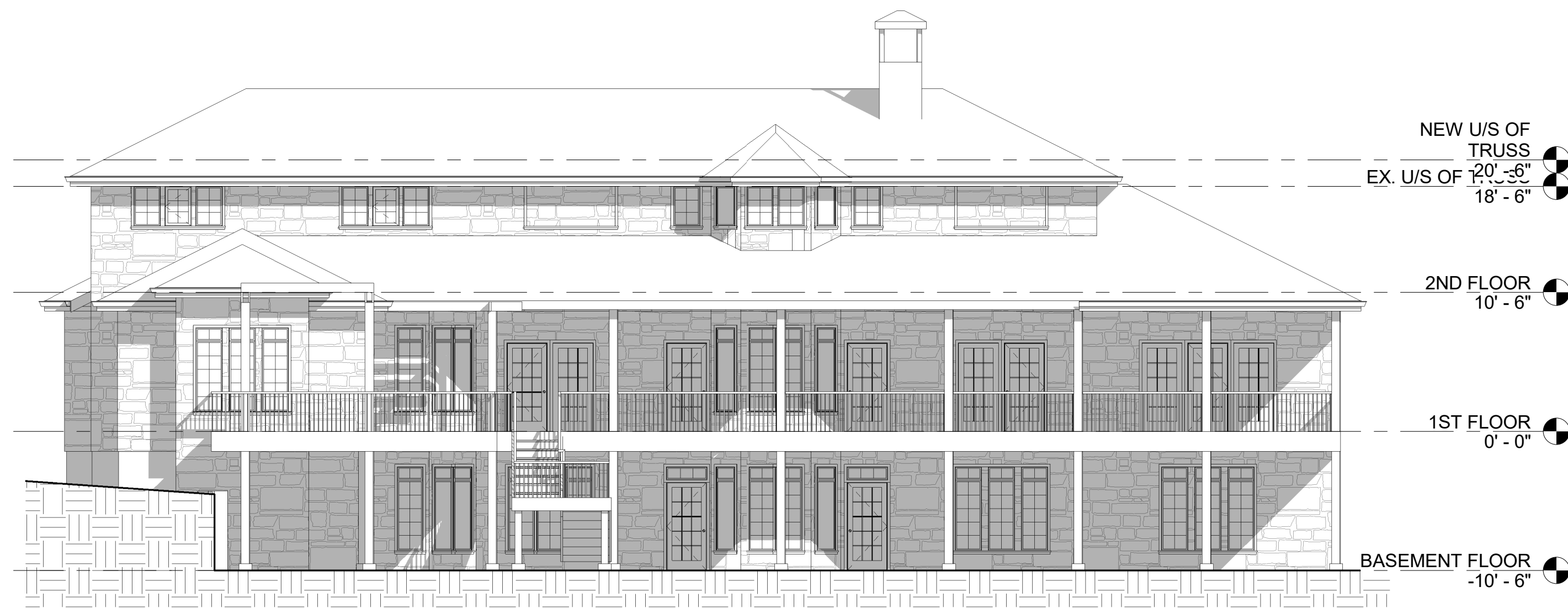
3 EXISTING WEST ELEVATION 1/8" = 1'-0"
