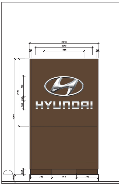
3 HYUNDAI PYLON FRONT/BACK ELEVATION SCALE 1:20
