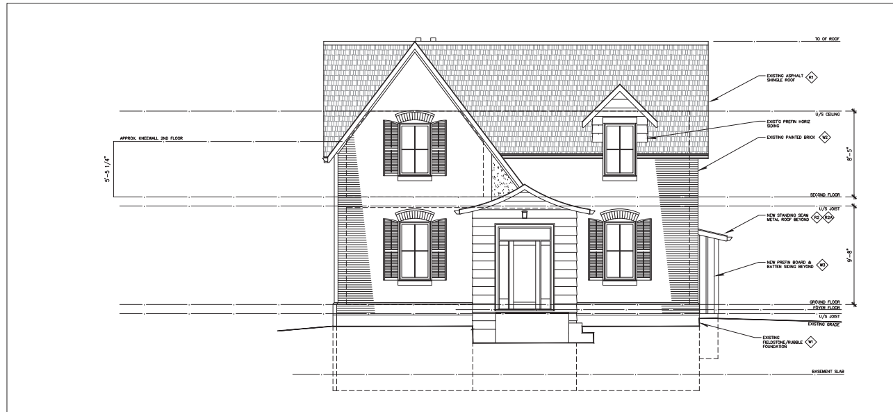
1 WEST ELEVATION - EXISTING TO REMAIN 1/4" = 1'-0"
