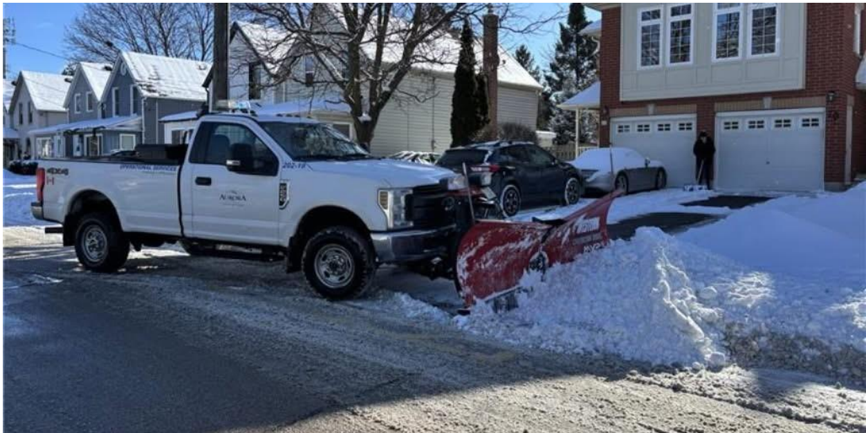
Figure 2: Shared driveway windrow removal reverse truck.
